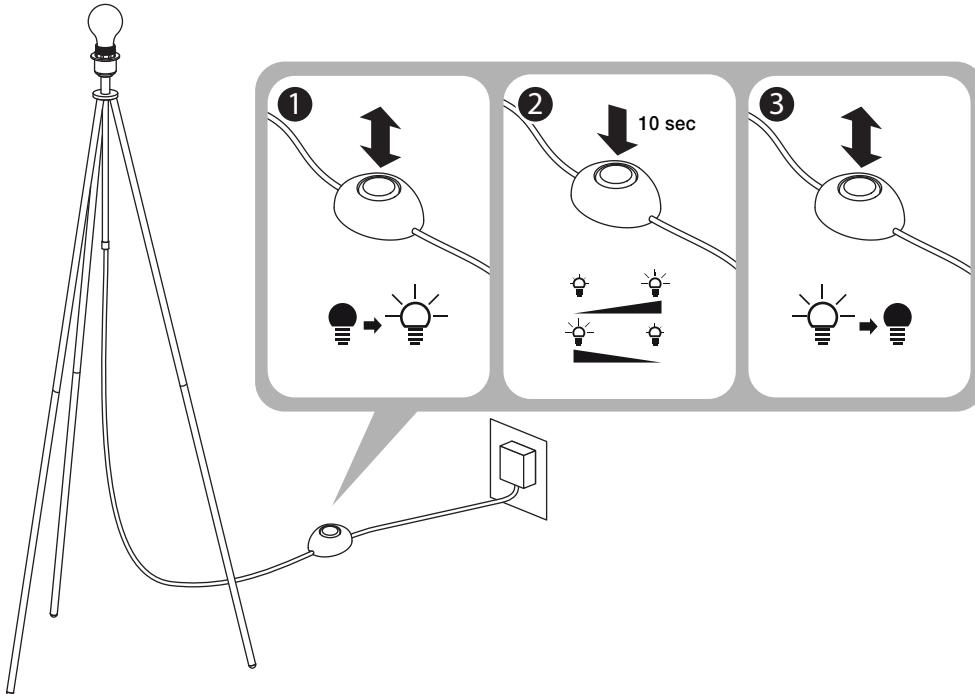
This Dimmer is designed to work with Dimmable LED Light Bulbs rated from 3W-100W. Results may vary if using Non-Dimmable or CFL bulbs or bulbs outside of this wattage range.
